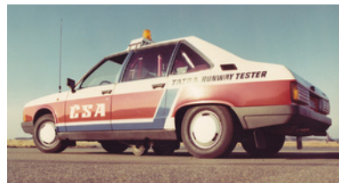
TATRA RUNWAY TESTER device for measuring surface roughness
