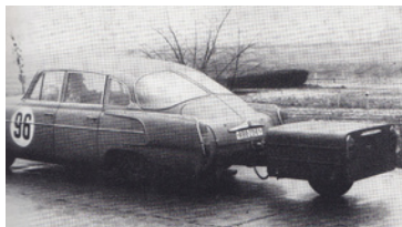
VÚD-1 device for measuring pavement roughness
