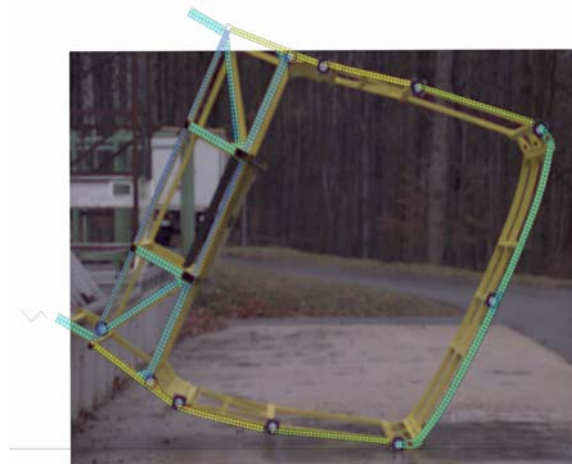
Figure 2: Highest deformation comparison (simulation vs. real test)
