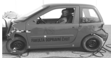
Figure 6: Deformation of SA5
