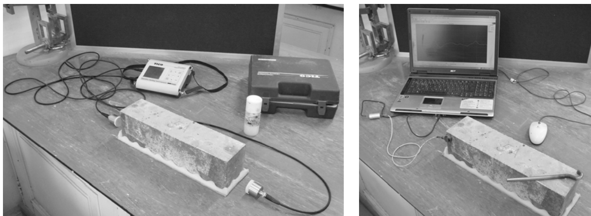
Figure1: Testing equipment – ultrasonic impulse method (left), resonance method (right)
