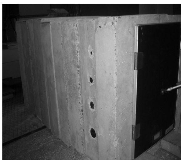
Figure3: Experimental path in Tomsk, ends of steel reinforcement apparent in the 2nd slab.
