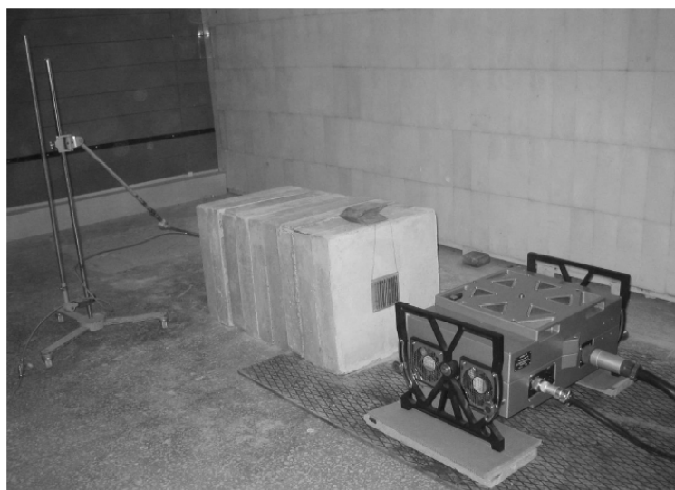
Figure 4: Scheme of the experiment in Tomsk – betatron MIB-7.5 and the experimental path.
