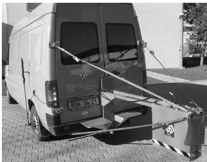
Figure 3: Configuration RoadScan 1.0 GHz mounted on a measuring vehicle.
