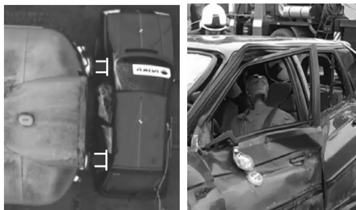
Figure 4: Detail of primary contact of the rail vehicle with the green Skoda Favorit (left), final position of a dummy after the crash test (right).
