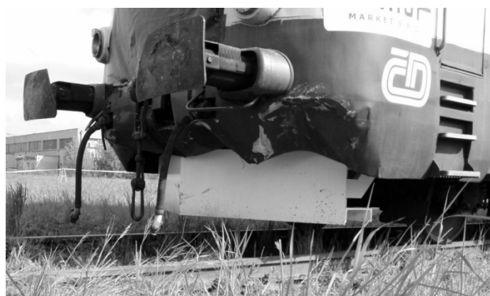
Figure 3: Detail of the front of the railway vehicle for the crash into a green Skoda Favorit and Superb.
