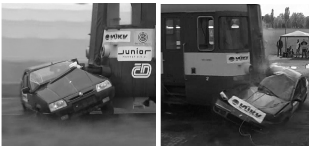
Figure 2: Detail of impact of the rail vehicle with the Skoda Favorit (left) and the Skoda Superb (right).
