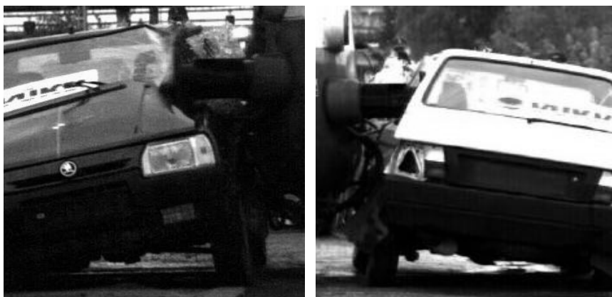
Figure 8: Contact of the head with the B-pillar, green Favorit, 75ms time from initial contact (left) and head contact with the B-pillar, white Favorit, time 85 ms from the initial contact (right).
