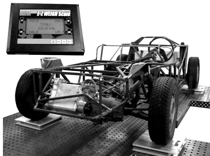
Figure 3: Illustration of how components are balanced on StudentCar Electric.
