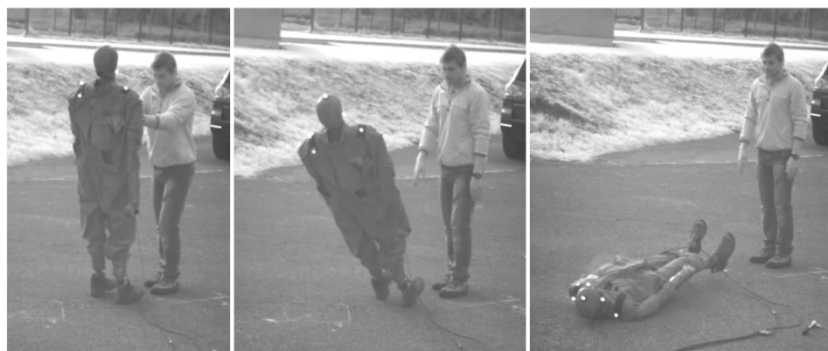
Figure 2: Backward fall of dummy after chest impact.
