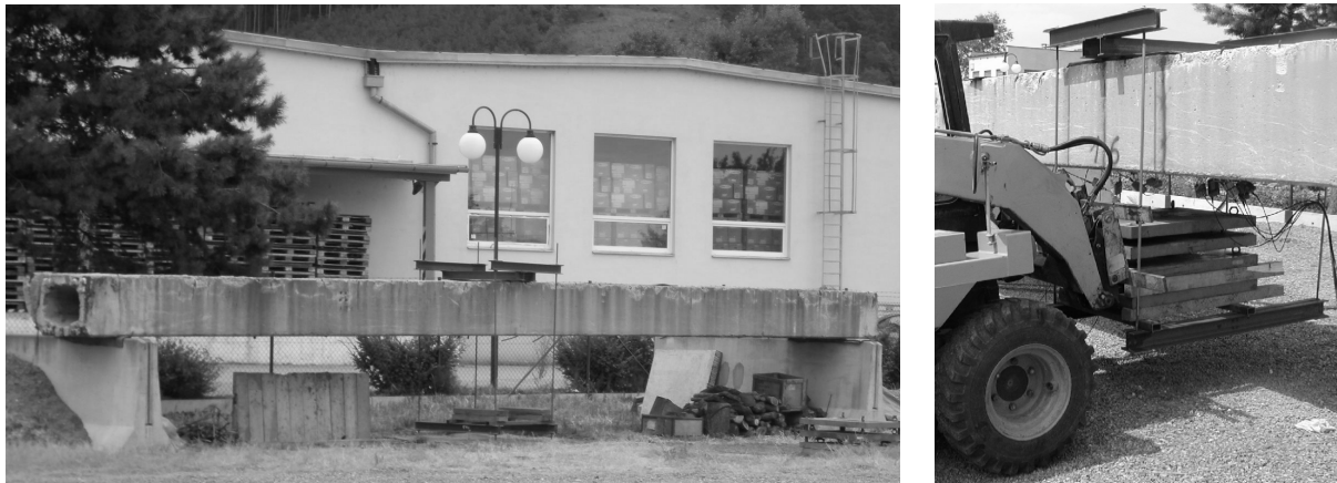
Figure 1: The girder with the loading frame (left), dynamic girder loading (right).
