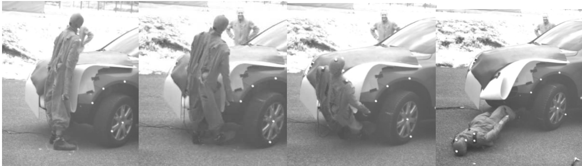
Figure 1: Backward fall of dummy after car impact.
