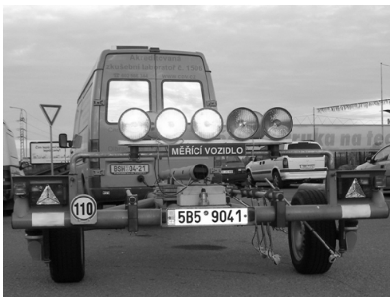
Figure 2: Placement of individual measurement microphones on CPX trailer.
