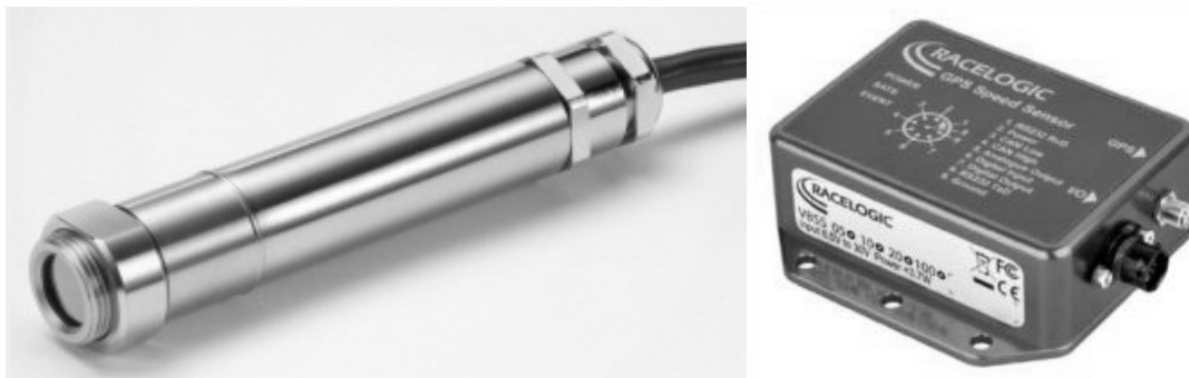
Figure 3: Non-contact infra-red temperature sensor CALEX and GPS module.
