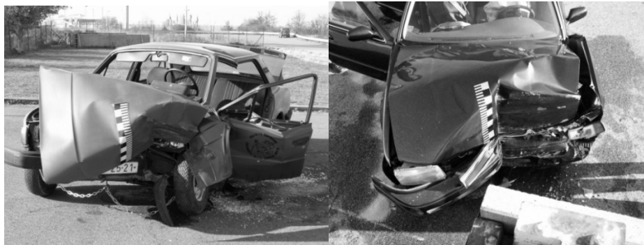
Figure 6: Technical condition of vehicle Škoda 120 (left) and Nissan Maxima (right) after collision.
