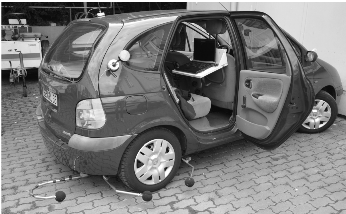
Figure 2: Eurovia measurement vehicle, CPX method.
